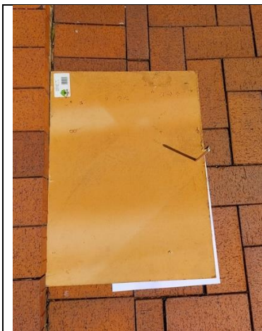
Figure 1: Shadow stick (a pencil) used to determine the altitude of the Sun
