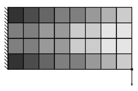
Each element in the macroscopic design uses a microstructure from our set.
